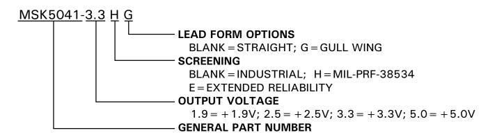
The above example is a +3.3V, MIL-PRF-38534 Class H regulator with gull wing leads.
